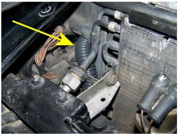
Route the tubing as shown across the front of the radiator, around the right side between the radiator and the inner fender, and to the Raptor.
