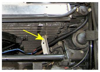
Before you mount the Raptor cooling unit, take the 1" convoluted tubing within your kit and push it into the hole in the side of the fan assembly. Also locate the wiring for this fan—it is red and black and bonded together. There are two of these wire sections in your kit. The one with the heavy wires are for the fans, the smaller one is used here on the Raptor fan. Attach the wires to the junction block on the side of the fan assembly now.
