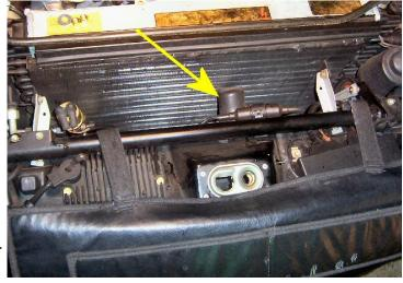
Take a moment now to remove that electric servo motor and unplug the wiring. Remove the mechanism, and affix the louvers in the wide-open position.
