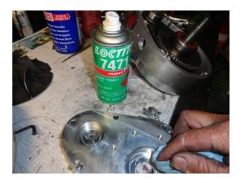
Apply loctite 515 to outer edges (only) of both bearings. Never put compound into holes in plate
