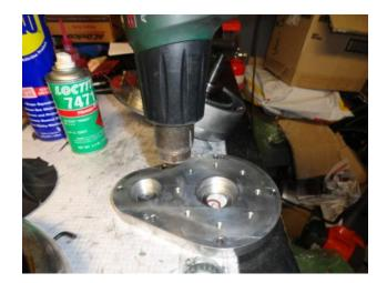
Use heat proof gloves, pick up plate and start it onto the small bearing while pushing it away from the large bearing, then push plate down onto large bearing and very quickly work the plate all the way down until it seats onto cowl. NEVER PULL IT ON WITH THE SCREWS
