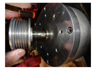
Restrain pulley and tighten nut by hand, never use impact wrench.
