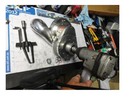
Remove drive pulley using a puller – sometimes heat may be needed for pulley to release from shaft easily
