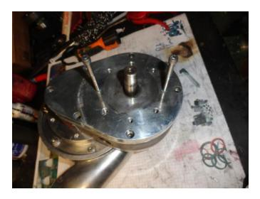
Use electric heat gun to heat upper bearing area for 60 seconds at maximum heat setting. Once heated then begin to screw the 2 screws in evenly until front cover is entirely removed
