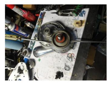
Now clean all belt fibres from all surfaces of the low speed pulley
