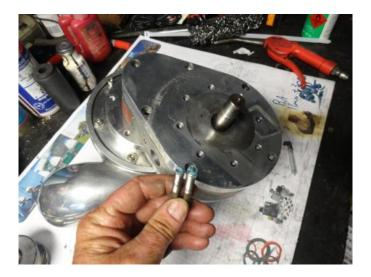
Take a torch and look into screw hole as shown, turn shaft until you see the peak of a pulley tooth at end of hole
