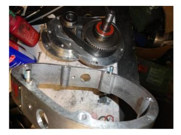
Using 7471 primer, clean outer edge/race of bearings and also bearing recesses in front alloy plate of transmission
