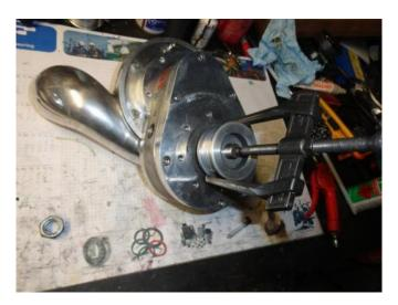
Remove key from shaft using side cutters, most efficient – lever key out
