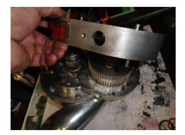
Turn supercharger over and heat rear section in approximate area of the low speed bearing, make the area hot to touch.
