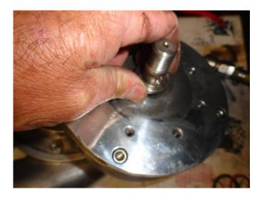
Loosen and remove the 6 socket headed screws from front of transmission
