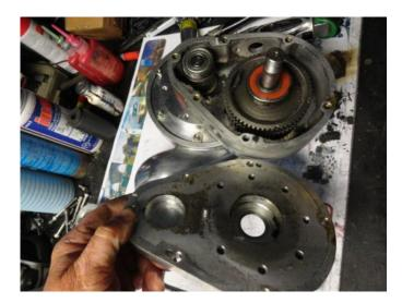
You can now remove the central cowl from the transmission, a few gentle taps with a rubber mallet will assist in loosening this part. The entire drive will now be exposed.
