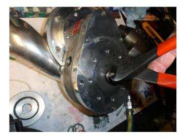
Remove pulley spacer - IF your charger has one, some pulleys have integral spacer
