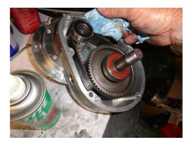
Bearing recesses being cleaned
