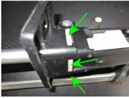
The liner is in place when all three of the tabs latch into the slots provided for them.
