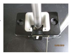
Re-install the hatch receiver in the car, with any spacers below it as it was before.
