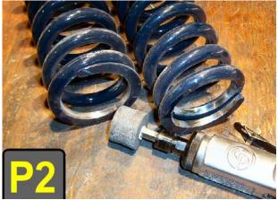
Picture P2 is to remind you to that your finished grind should be with a fine stone so as to leave no cuts or stress risers at the bottom of the spring.
