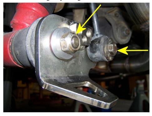
Tighten the lower drop-link bolt to 33 lb ft.
