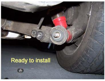
Install the new drop-link mount as shown below.
