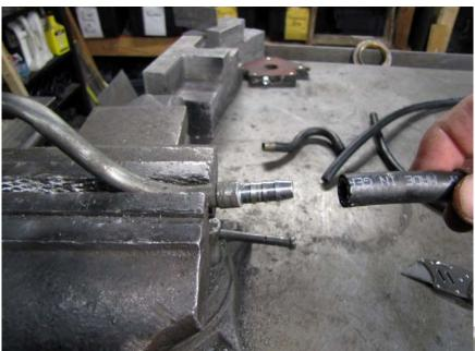
Push on the new fuel line onto the barbed section.
