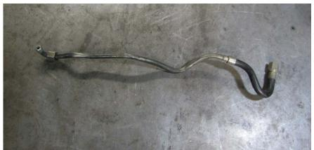
This is typical of the steel-andrubber fuel line that you will find on your Porsche. The steel elements are fine, but the rubber section needs to be replaced.
