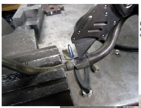
Use a razor to slice the remains of the rubber hose down to the fitting.
