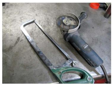
You will want to use a hacksaw or a metal cutting wheel to remove the ferrules on the ends of your old rubber hose.
