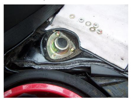
Use a screwdriver and pry up the dust cover and set it aside. It will not be going back on.
