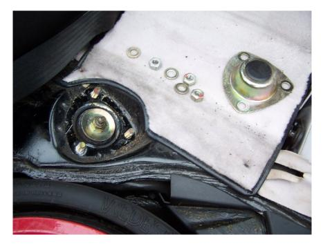
Place the seat belt mount over the shock bolts as shown....
