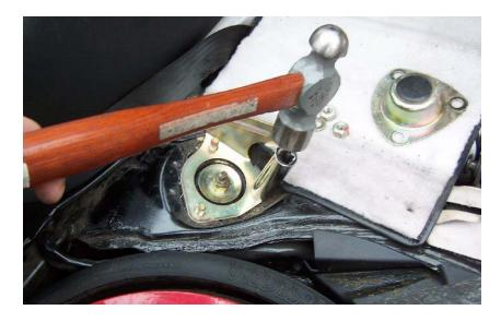
Re-install the washers and the nuts, and tighten.
