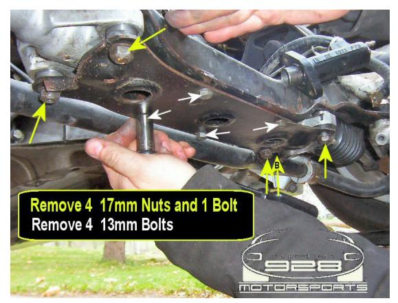
Pull down the Reinforcement Plate and set it aside.
