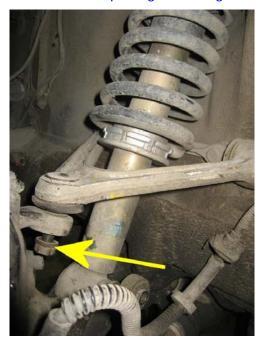
Remove the two nuts on the inner fender that secure the a-arm to the frame. They are just outboard of the exhaust manifolds.
