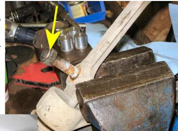
NOTE: the mounting cross-bar is not symmetrical. You must insert the mounting studs into the cross-bar from the side with the small relief out to the side with the large relief.
