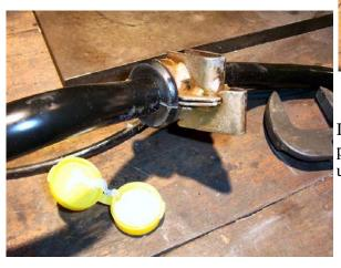
Install a collar on each side of the bushings to prevent them from backing out. Snug the collars up, but do not fully tighten yet
