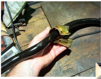
Close the clamshell and latch it with a large slip-joint pliers as shown.
