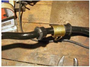
Wrap the new polyurethane bushings over the sway bar now—one on each side of the clamshell.
