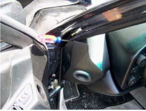
We've learned that one of the easiest ways to route the wires from behind the dash to the gauges is to open the drivers side door and slide your screwdriver tool behind the dash just below where the A-pillar meets the fender. Push a screw driver through the gap where they meet from the outside and it will be able to be seen on the inside if you lie on your back by the pedals. (Put the seat all the way back for comfort).
