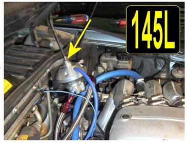
Make several "pulls" on a country back-road, turning the brass thumb screw under the BLUE arrow until the orange needle on the air/fuel gauge holds steady at Wide-Open Throttle right to red-line.
