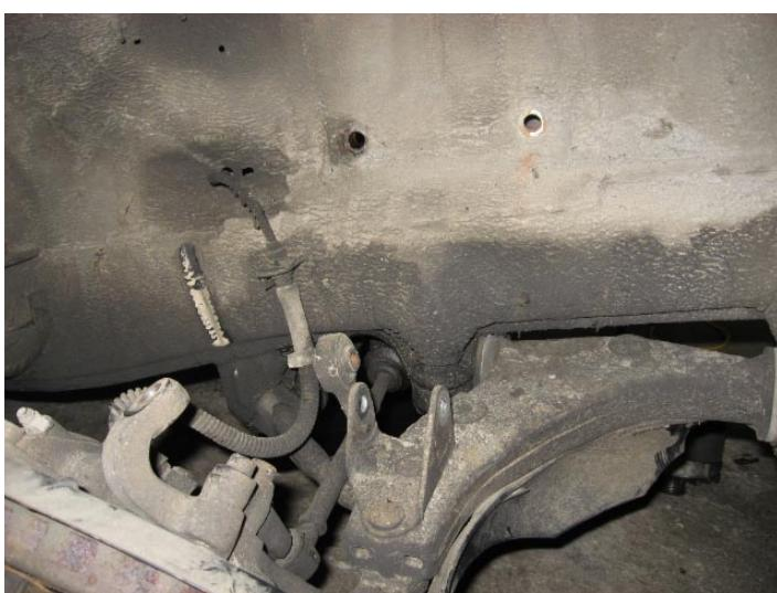
Remove the bolt that goes through the bottom of the shock absorber, and the 3 bolts that secure the shock tower to the fender at the top. Remove the shock, spring, and upper a-arm all as one piece.
