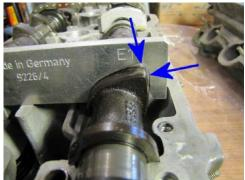
The German tools are marked "E" for the Intake cams, and "A" for the exhaust cams. 928 Motorsports makes these tools in English as well, and they are marked "Intake" and Exhaust" for your ease of use.
