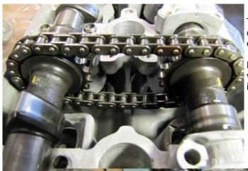
These photos show 7-and-a-half links of the cam drive chain, and how that appears when checked with the cam profile tool.
